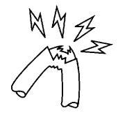
Do not damage, forcibly bend, pull, distort or bind the power cord. Do not place heavy objects on it, or allow the power cord to be caught or pressed.
